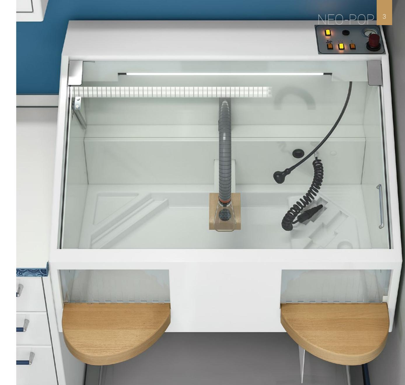
The box with suction system prevents the dispersion of powders in the surrounding during the work of roughing down or finishing. It is equipped with external control panel and tempered glass protection.
